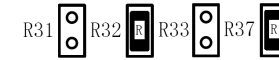
(c) R32, R37 short circuit, CW/CCW mode effective at LOW level (The fixed level)
