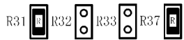
(a) R31, R37 short circuit, PUL/DIR mode DIR HIGH for Positive Direction
