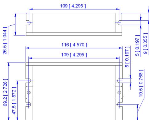
Figure 1: Mechanical specifications
