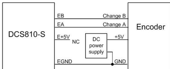
Figure 4: Using external DC power supply to supply the encoder
