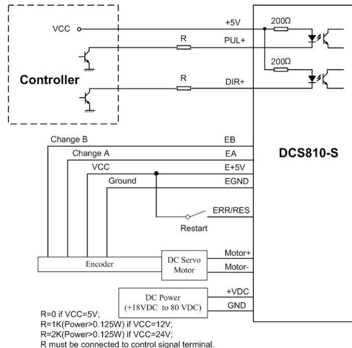
Figure 6: Typical connection (Open-collector control signal and single-ended encoder.)
