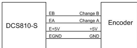
Figure 3: The DCS810S supplies the single-ended encoder directly
